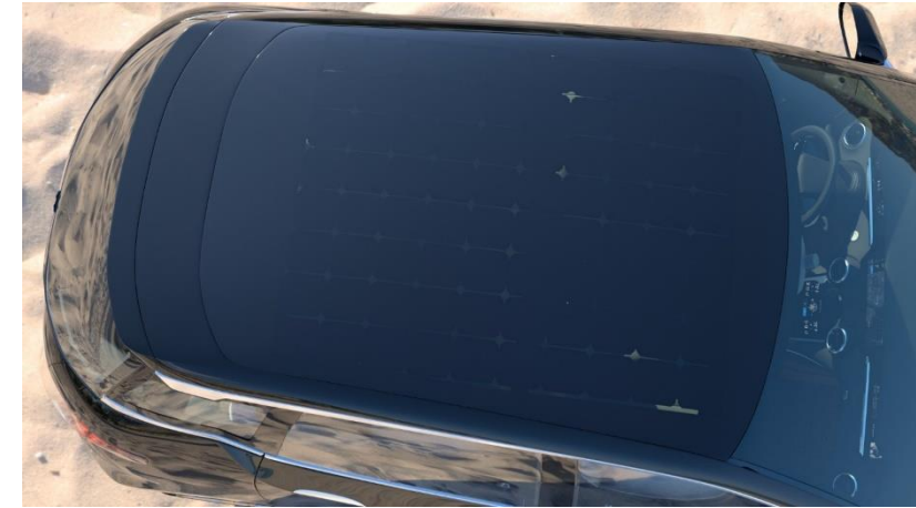
With back contact (xBC) solar cells
